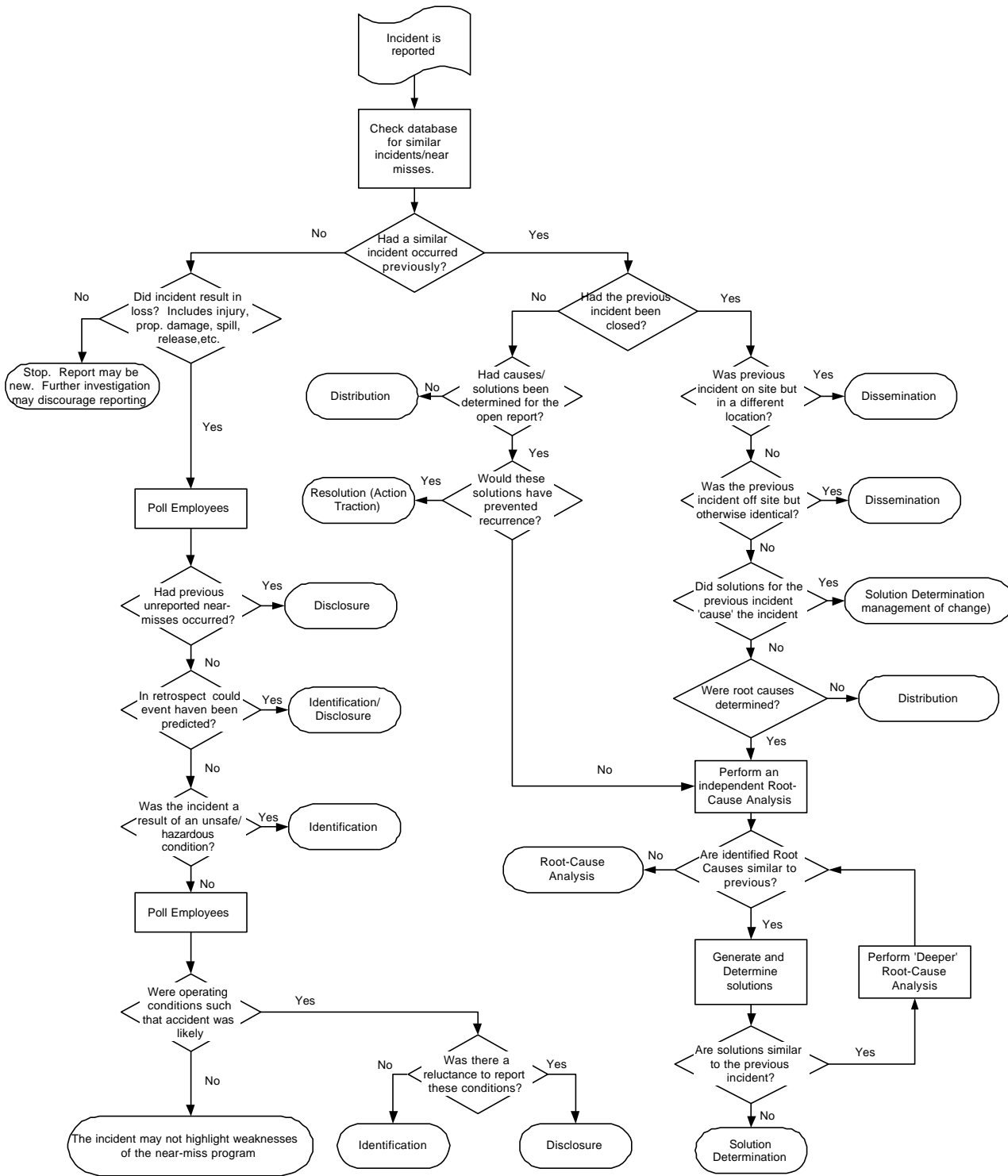
Figure 9. Identifying Potential Weaknesses in Near-Miss Management Program Stages Based on Repeat Incidents or Accidents (potential weaknesses shown in ovals)
