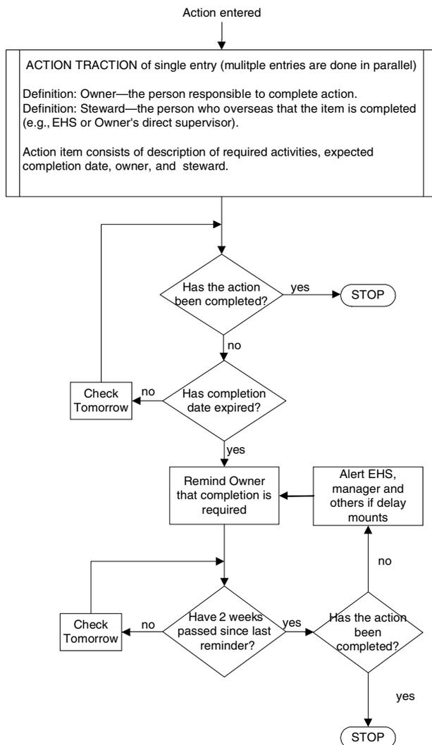
Fig. 8. Action-traction algorithm.
