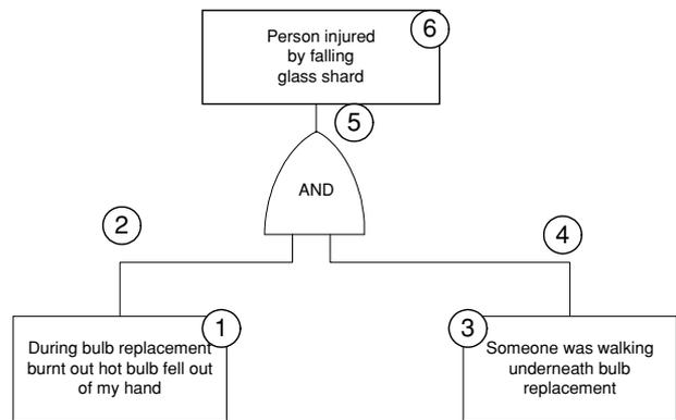
Fig. 6. Near-miss fault tree for bulb-breaking incident (circles 1–6 represent leverage points for corrective actions; see Solution Identification).
