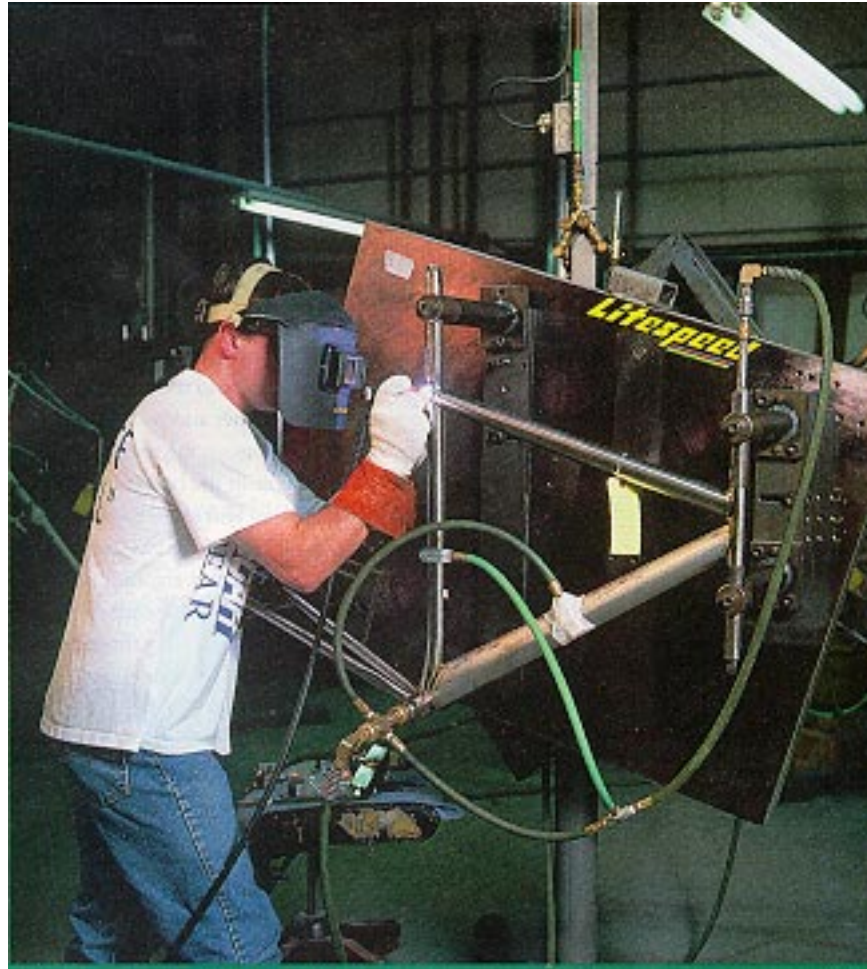
Exhibit 5: Conventional hard fixture for positioning tubes for welding.
